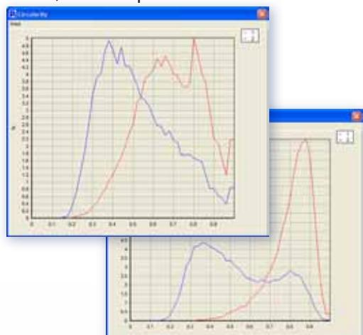
Most particle size analyzers assume particles to be spherical without taking into account other critical shape factors. In the above example, the difference in two samples, similar in size when assumed to be spherical, are clearly demonstrated in overlays of both circularity and smoothness. Only a particle shape analyzer can render such critical shape information.
