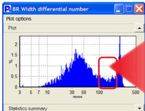
The Particle Insight allows the user to have a true analysis of all dimensions of the particles. In addition, the user is able to selectively see each particle that created a certain area of any shape histogram.
